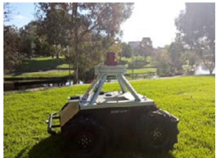
From our physiological experiments, we develop neuro-inspired, autonomous robots. This ground vehicle autonomously chases moving objects, even amidst distracters.
