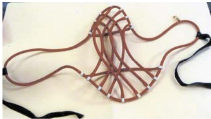
THE STRING HAT WAS PLACED OVER THE HEAD TO HOLD THE ELECTRODES IN PLACE. CLIP ELECTRODES WERE PLACED OVER THE EARS AND DISC ELECTRODES WERE PLACED ON THE MASTOID PROCESSES BEHIND THE EARS
