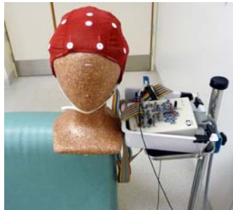
A CAP WITH ELECTRODES AS CURRENTLY USED AT THE QUEEN ELIZABETH HOSPITAL. THE MULTI-COLOURED LEAD CONNECTS THE ELECTRODES WITH THE RELAY AND TO THE (HEAD) CONTROL BOX (ABOVE RIGHT)
