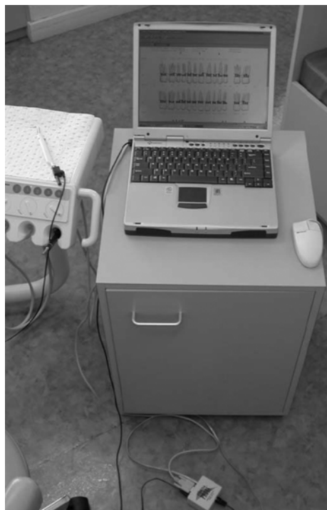
Figure 2. The Florida Probe, consisting of a probe handpiece, computer interface which is connected to a computer laptop, power supply, foot controller and the probe handpiece.
